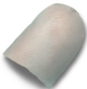
Figure 1: A wafer-thin silicon dummy of a fingerprint
